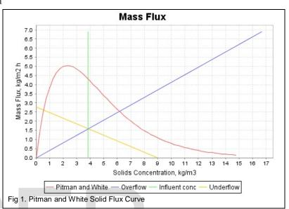
The state point analysis used to predict the solid behaviour in the tank was examined based on the four criterions applied to settling clarifiers. As described by the Water Research council, criteria I (a) and II are the most common and criterion III and IV by the German ATV guidelines.
